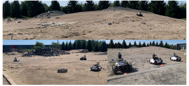
FIGURE 1. Multirobot experiments at the CSA Mars Yard. In our experiments, three robots simultaneously explored the simulated Martian terrain. The robots collaborated through peer-to-peer communication to map the environment and localize themselves within the landscape, demonstrating the effectiveness of our C-SLAM system in a challenging, planetary analogue setting.
