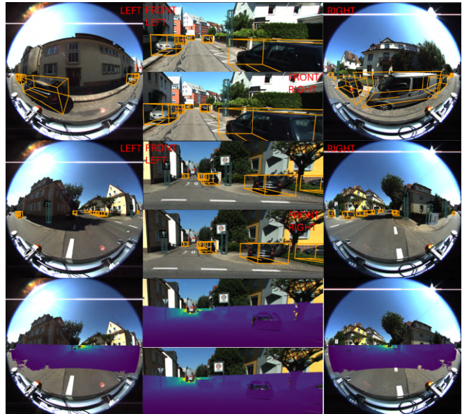
Fig. 1: Qualitative detection results on KITTI-360 mixed camera configuration. 3D bounding box and point cloud rendering overlaid on pinhole and fisheye images. The visualization is created with a customized nuScenes devkit. Our method successfully handles the severe radial distortion in fisheye cameras while maintaining consistent detection accuracy across different camera types.
