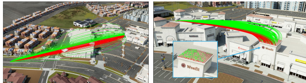
Fig. 6: Generated navigation and interaction trajectories for the example mission: landing on the red roof of the Weefit building. Green lines represent feasible navigation and interaction trajectories, and red lines denote failed attempts. Sampled point clouds are displayed within the blue box, with red dots indicating failure landing points.
