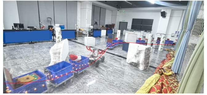
Fig. 5: Part of the indoor experimental area. Tractor-trailer robot is traversing complex indoor environment.
