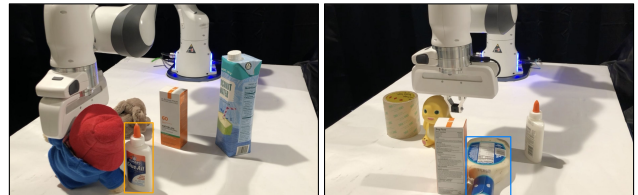
Fig. 8: Examples of real-world failures generated by IMPACT. In the left image, the robot gets stuck on the toy bear while reaching the target glue bottle. In the right image, the robot does not rotate the gripper in time and collides with the ranch bottle.
