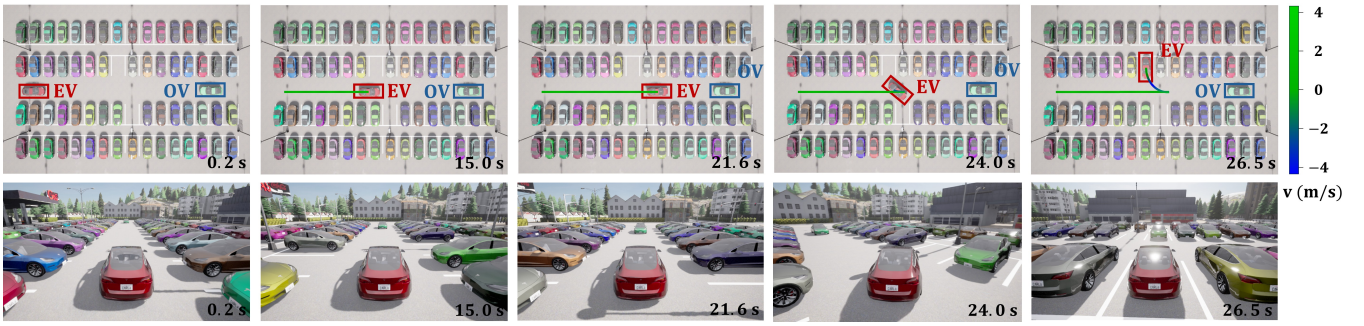
Fig. 4: Key frames of the interactive parking process under task type ii on target slot S_{15} . The top section presents a top view, in which the parking trajectory of the EV is represented by a solid line whose color varies according to speed. The bottom section provides a third-person perspective view of the EV.
