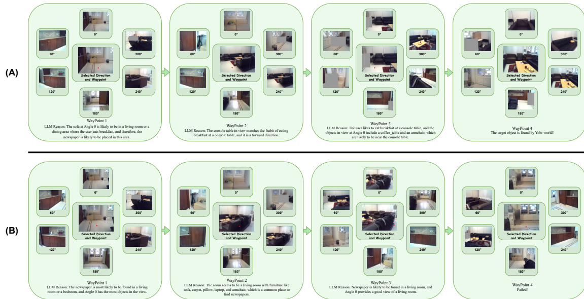
Fig. 4: A Case Study in The Small Environment We show the waypoints and LLM reasoning results from one experiment. In this experiment, a newspaper, as a target object, is deliberately obscured by our laptops. The agent is told about the user’s habit of enjoying breakfast on the console table while reading the newspaper. The red squares represent the waypoints chosen by PixelNav. (A) The habit level is Retrieval. The agent first identifies the room where breakfast is served, then determines that the newspaper is nearby based on the console table in the field of view, and eventually finds the target. (B) The habit level is None. The agent can only use common sense to determine that the newspaper might be in the living room or bedroom, and then search aimlessly through the living room. In the end, the agent fails to find the target object
