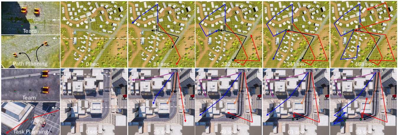
Fig. 5. Qualitative results illustrating the generalizability of CoPCS in unseen environments. The large-scale suburban and urban maps are not used during training and also contain variations in starting points and road network layouts. In the top environment, a 2-UAV and 2-UGV team is required to visit 15 tasks, while in the bottom environment, a 4-UAV and 2-UGV team is required to visit 15 tasks.
