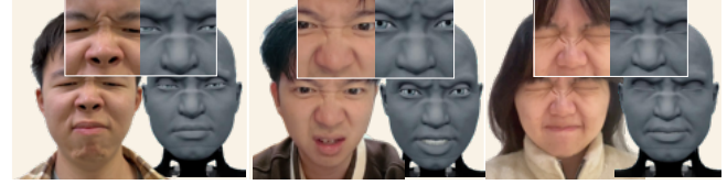
(b) With motion transfer module fine-tuning, nose wrinkles are successfully transferred to the robot face.
