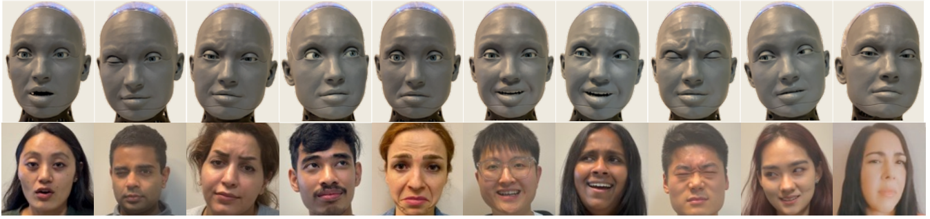
Fig. 5: Real-world examples of humanoid robots performing realistic facial expression imitation.
