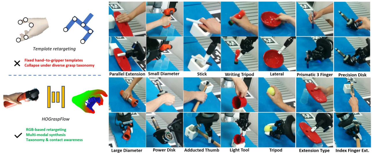
Fig. 1: Grasp demonstrations for parallel jaw grippers via HOGraSPFlow
