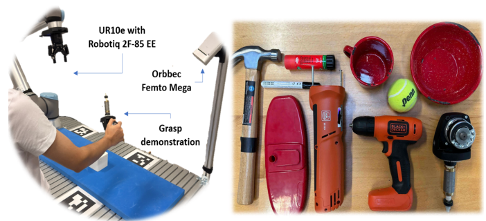
Fig. 6: Experiment setup (left) and objects in real-world experiments (right). The hammer, marker, mug and bowl are from the HOGraspNet ( In dist. ), others are OOD ( Out dist. ).
