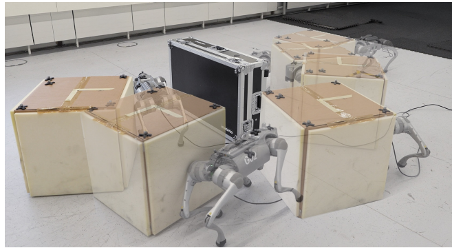
Fig. 1: Robot loco-manipulation in the real world enabled by CAIMAN. The quadruped maneuvers a box around an obstacle to reach a target position.
