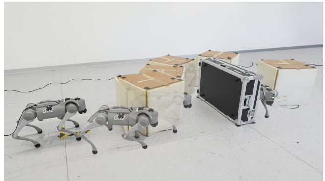
Fig. 9: Snapshots from hardware deployment for the single object and single wall tasks. The mass of the box is 5.5 kilograms with a dimension of (0.55, 0.55, 0.5) meters.
