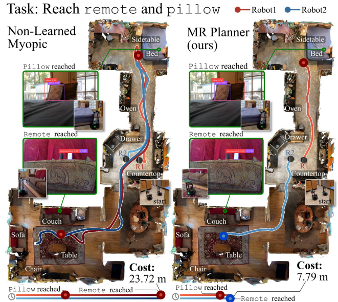
Fig. 1. Planner Comparison in Home Environment: Two robots are tasked to reach remote and pillow with the exact locations of these objects unknown. A myopic approach searches the nearest locations first, until the task is completed, leading to poor behavior. Our approach utilizes learning with a model-based planning framework to best guide the robots for efficient task completion. See further discussion in Section VII.
