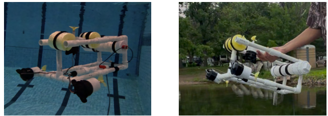
Fig. 1: The Jar Jar ROV in a pool (left) and lake (right) with the attached water quality sensor pod. With the three-thruster configuration, the ROV can move in three axes, left-right ( x/yaw ), up-down ( y/heave ), and front-back ( z/surge ).
