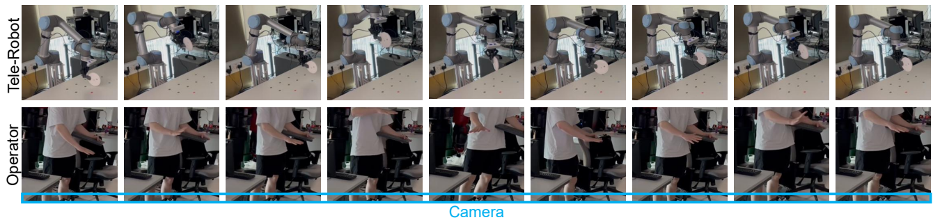
Fig. 9: Qualitative demonstration of teleoperating the UR5 robot with OAT. The robot grasps a plate to better illustrate end-effector rotation. The operator’s right hand, captured by a ground-level camera, is retargeted to control the robot, while the left hand operates a keyboard to trigger the start and termination of teleoperation.
