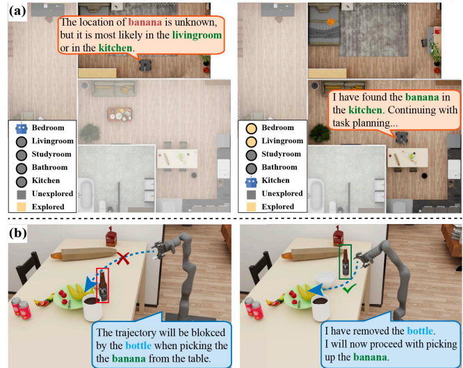
Fig. 1: An example illustrating the challenges of integrating exploration and sequential manipulation: (a) Robots must prioritize potential exploration locations and balance exploration with manipulation tasks to execute efficiently. (b) The robot needs to engage in situated planning to handle unexpected situations.
