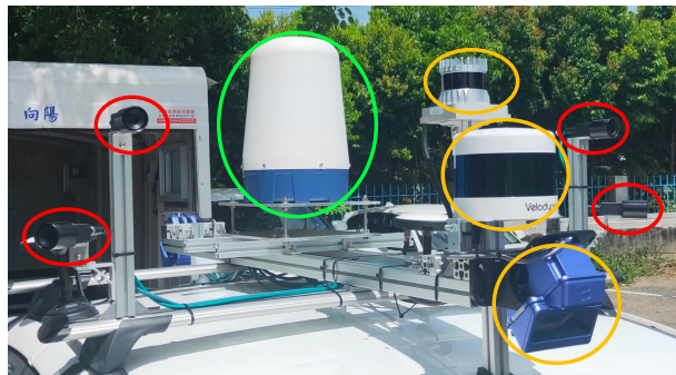
Fig. 5: Sensor setup for the data collection car in the ITRI dataset. The green circle highlights the scanning radar (Navtech CIR504-X), and the orange circles indicate LiDARs, from top to bottom: Ouster OS1-128, Velodyne VLS-128, and Baraja Spectrum-Scan. Red circles indicate four cameras.
