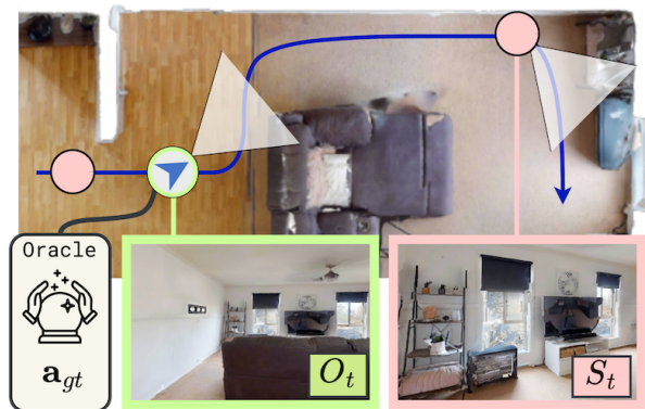
Fig. 4: Training data collected from the simulator - oracle actions \mathbf{a}_{gt} that control the agent, agent observation O_t , and subgoal image S_t .
