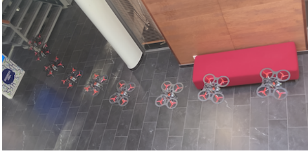
Fig. 7: Drone trajectory relative to \mathcal{M} when controlled by FAINT. The drone successfully reached the goal on the left trajectory ( RMSE 1.07 m), but missed it on the right ( RMSE 1.42 m).
