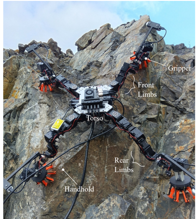
Fig. 1. Limbed climbing robot scaling an unstructured terrain [6].
