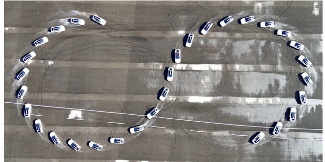
Fig. 1: Demonstration of our autonomous drifting control algorithm in a production vehicle performing figure-eight drifting on a surface with mixed wet, damp, and dry conditions. [9]
