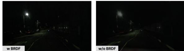
Fig. 6. Comparison of BRDF-constrained and direct evaluation of ASGs. BRDF-constrained ASGs produces more physically realistic lighting and construct overall better quality rendering than direct evaluation.
