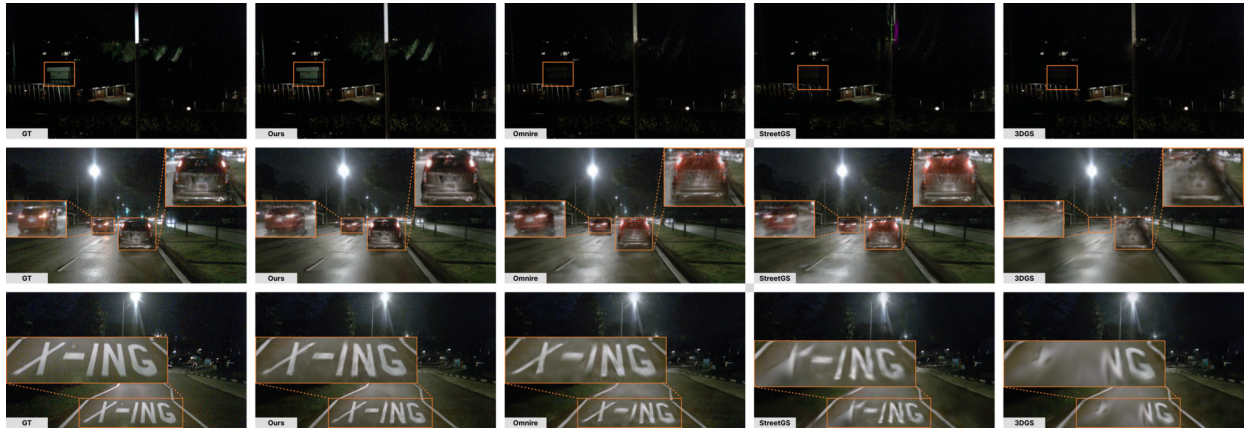
Fig. 3. Qualitative results from the nuScenes Dataset. Columns show results from GT, Ours, OmniRe, StreetGS, and 3DGS, respectively. Fine-grained details such as traffic lights, vehicles, and trees are highlighted to illustrate differences in reconstruction quality.
