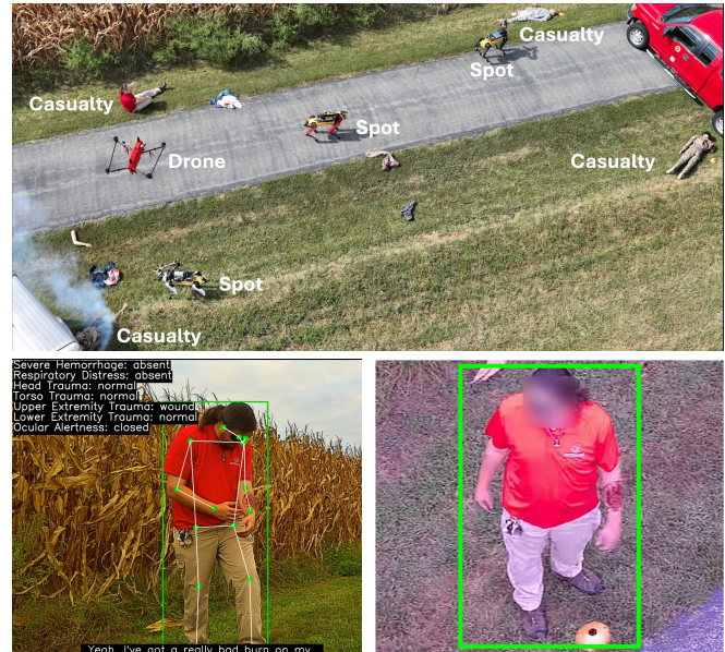
Fig. 1: (Top) Three customized Boston Dynamics Spots and one custom drone performing medical triage of casualties in simulated mass-casualty incident. (Bottom) Spot and drone injury assessments of same casualty.
