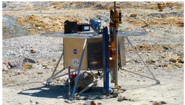
Fig. 1. Robotic drill lander concept in Spain in 2017
