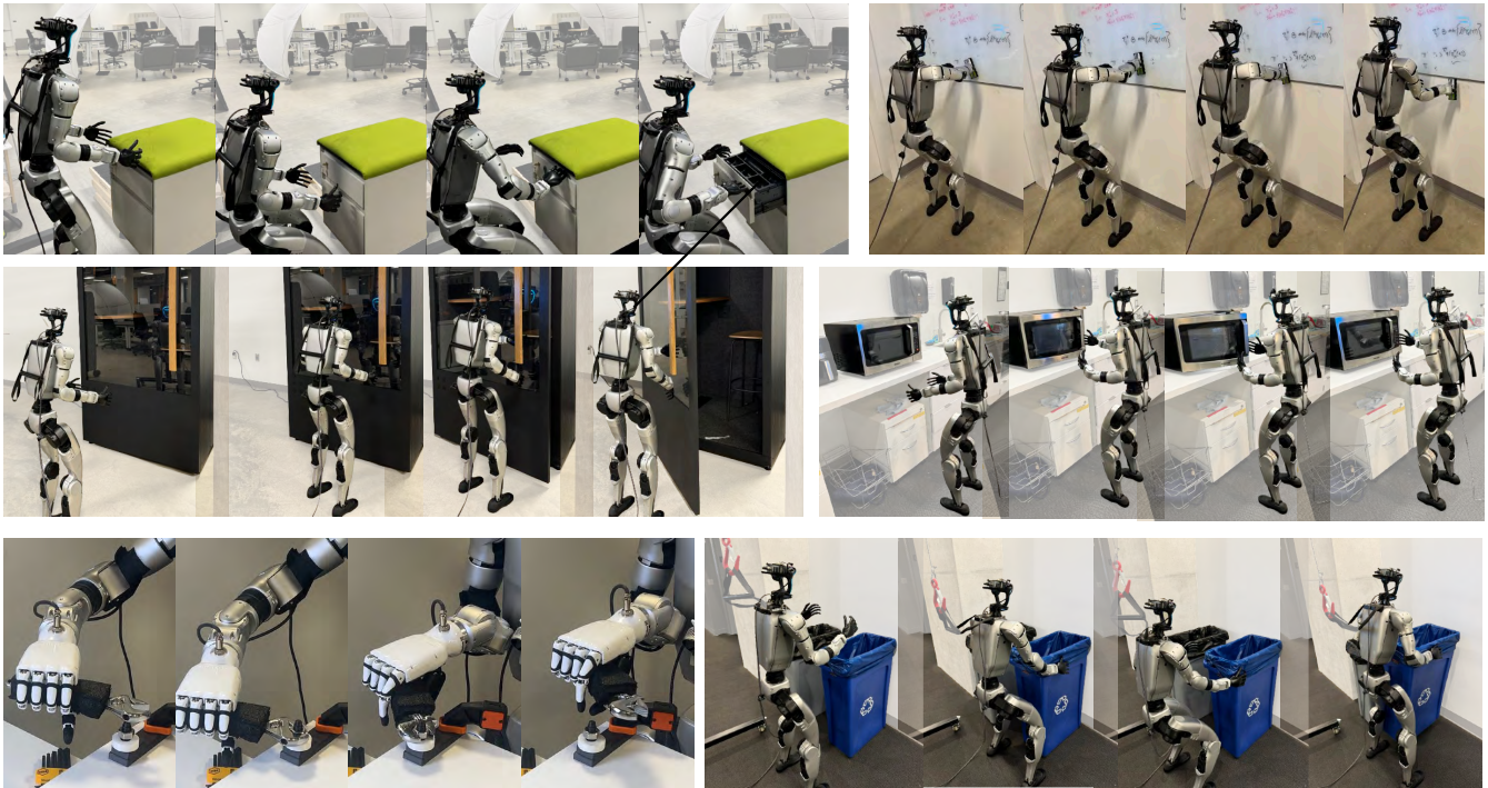
Fig. 1: Rolling out HMC for contact-rich tasks on a humanoid robot. Compared to naïve position-only policies [5, 26], HMC designs a blending interface (HMC-Controller) that dynamically balances the torques from position tracking and force-aware controllers for contact-rich tasks. Using a heterogeneous architecture, HMC-Policy trains on both large-scale position-only data and fine-grained force-aware demonstrations. (Shown tasks: opening a wheeled cabinet; wiping a whiteboard; pulling open a door; opening a microwave; tightening a nut and lifting a trash can.)
