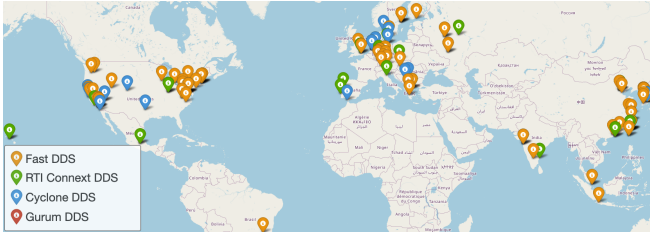
Fig. 8: Global exposure map of DDS-based systems detected by our Internet-wide scan, colored by implementations supported by ROS 2 Humble and Jazzy. Deployments were found across the Americas, Europe, and Asia, highlighting the real-world attack surface of public ROS 2 systems.
