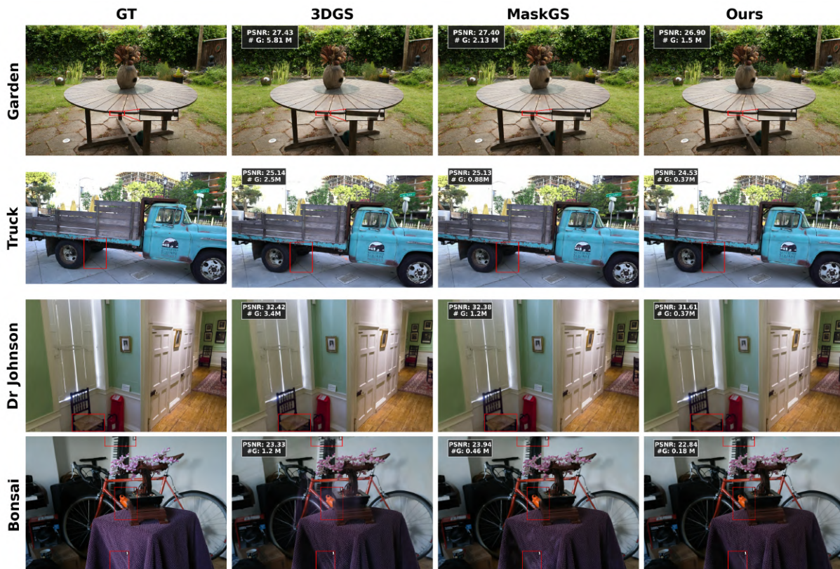
Fig. 4. Qualitative comparison of our method with 3DGS and MaskGS. For each scene, we report PSNR (dB, \uparrow ) and #G (M, \downarrow ), where #G denotes the number of Gaussians in millions. Regions with differences are marked in red boxes.
