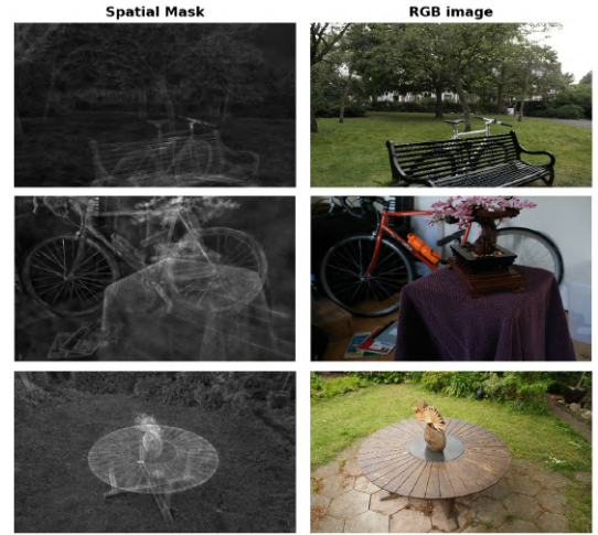
Fig. 3. Spatial mask F(x) rendered via Eq. (4) (left) alongside the RGB image (right). High intensities correspond to small per-Gaussian contributions \alpha_i(x)T_i(x) , highlighting occluded or faint structures.
