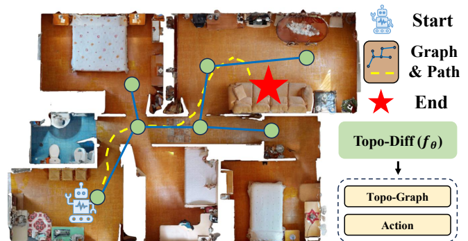
Fig. 1: An example of DIPP, our framework for ObjectNav framed as a dual objective. Our core diffusion model, Topo-Diff, synergizes navigation and mapping by simultaneously generating a structural topological graph (blue) and a goal-oriented action plan (realized as the yellow path). This synergy enables the agent to build an abstract map while efficiently navigating from the start to the goal (red star).
