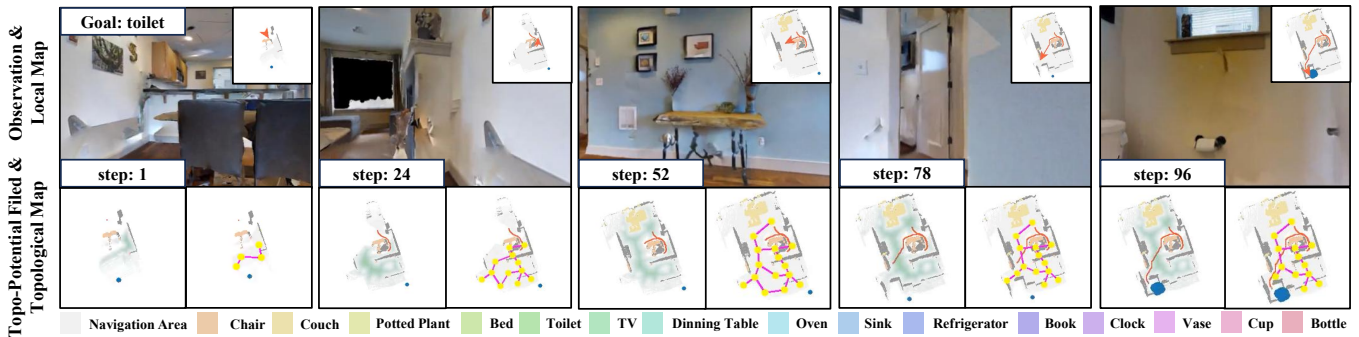
Fig. 5: A qualitative visualization of navigation with DIPP, tasked with finding a ‘toilet’. The main images show the agent’s first-person view, with top-right insets displaying the local map and agent trajectory. The bottom row visualizes our model’s core outputs: the generated Topological Potential Field ( \hat{U}_{\text{topo}} ) and the resulting topological graph. (Steps 1-52) During initial exploration, our model generates a dynamic Topological Potential Field ( \hat{U}_{\text{topo}} , green heatmaps), whose peaks directly guide the placement and adjustment of new topological nodes (yellow dots). (Steps 52-96) The value of this synergy becomes evident at the hallway junction (step 52), where the agent leverages the accumulated topological graph—itsself a product of the potential field—to make an informed decision. This demonstrates our framework’s core feedback loop, where intelligent map construction provides the global awareness for efficient navigation to the goal.
