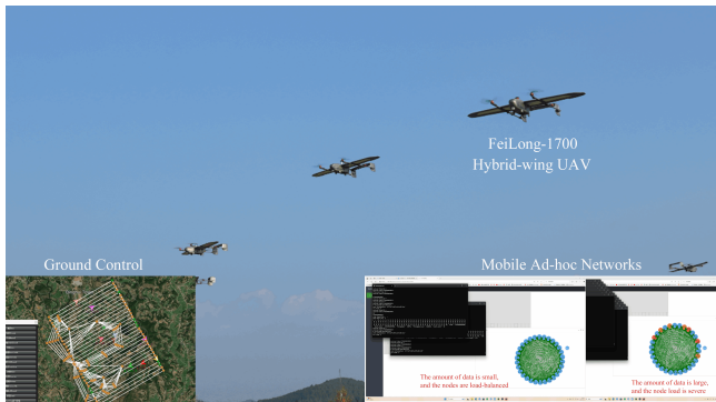
Fig. 6. Fei Long-1700 UAV swarm executes distributed task allocation algorithm in the search and rescue task.
