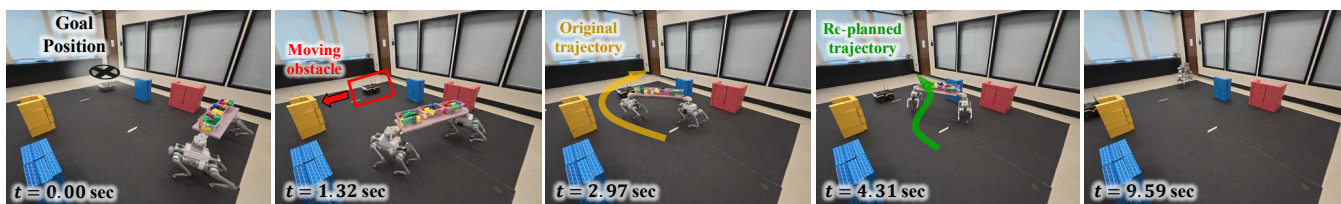
Fig. 7. CQTD handling a dynamic scene containing a moving obstacle by periodically re-planning. Originally intending to cross in front of the obstacle, the robot team instead crossed behind it.
