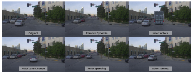
Fig. 8. GenRe+ can support diverse variants for reactive log replay, such as dynamic actor removals, actors insertions, and actors manipulation.
