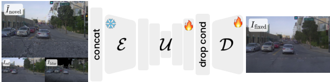
Fig. 3. 2D neural fixer ( FNet ) overview. FNet takes a 3DGS-rendered view \tilde{I} , conditions on the reference image I_{\text{ref}} and the rendered LiDAR map I_{\text{lidar}} , and produces the fixed image I_{\text{fixed}} . We fine-tune FNet from the pre-trained single-step diffusion model SD-Turbo [23].
