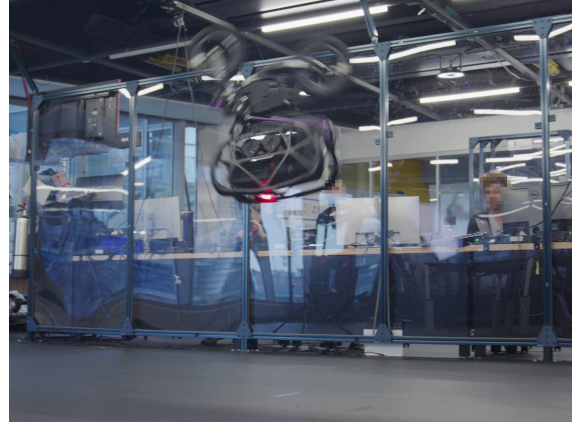
Fig. 1. UMV executing a front-flip learned via Iterative Motion Imitation .
