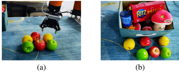
Fig. 5. (a) Physical robotic arm AUBO-i5 with realsense D435 depth camera and DH AG-95 parallel-jaw gripper. (b) Various objects we used for experiments.
