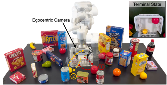
Fig. 8: Real-world setup mirroring the sequential manipulation task from simulation. Our policy is transferred from simulation to the real robot in a zero-shot manner and completes the task.
