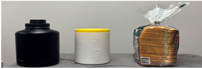
Fig. 4. Target objects to be tested. Object 1 (water bottle, rigid and heavy), Object 2 (plastic wet wipes container, medium stiffness), and Object 3 (bag of bread, soft and deformable).
