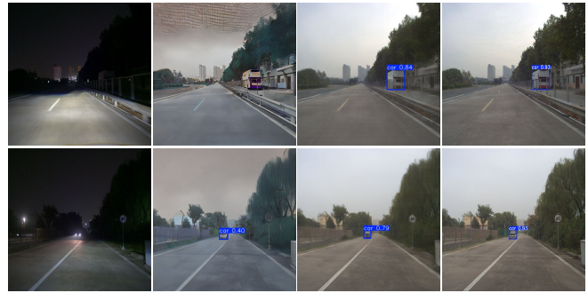
Fig. 8: 2D detection errors on nighttime images can be reduced after low-light enhancement. (a) and (d) are night-day paired data of DarkDriving dataset.
