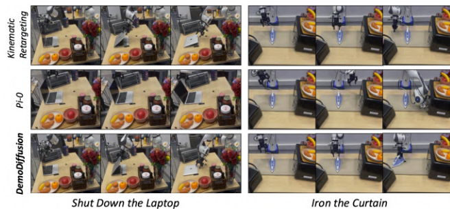
Fig. 6: Qualitative comparisons for real-robot manipulation. Rollout progressions (start, intermediate, final frame) for two tasks. Kinematic retargeting (top) produces plausible motion but loses contact before completing the task. Pi-0 (middle) performs general reaching but fails to manipulate the correct object. DemoDiffusion (bottom) reaches the object and maintains contact through task completion. See project page for full videos.
