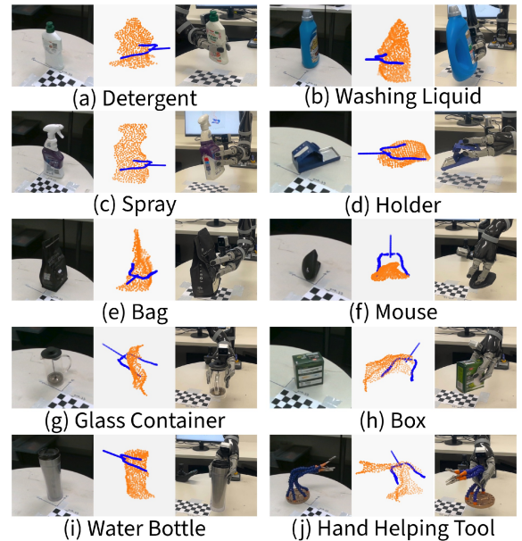
Fig. 9: Illustration of the real experiment. For each object: left—camera view, middle—scanned point cloud with predicted grasp, right—KG3 gripper executing the grasp.
