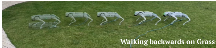
Fig. 3. Real-world deployment of quadruped policies trained with minimal expert data. The upper left shows expert demonstration. Using the same data, behavior cloning (bottom left) fails to walk, whereas our Latent Variation Regularization (LVR, right column) produces stable forward and sideways walking. LVR further shows robust performance, such as walking backwards on grass by training on data from walking backwards on flat indoor ground.
