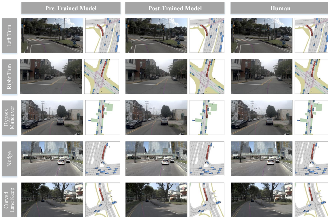
Fig. 4: Qualitative results of various scenes between the pre-trained and post-trained model. The red rectangles in the BEV figure represent the future waypoints of the ego agent. Others represent agents in the current timestamp.
