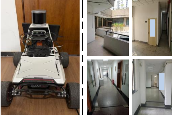
Fig. 4: The figure shows the unmanned vehicle equipped with a 32-line LiDAR sensor (left) and the indoor experimental environment containing narrow corridors and other indoor scenarios (right).
