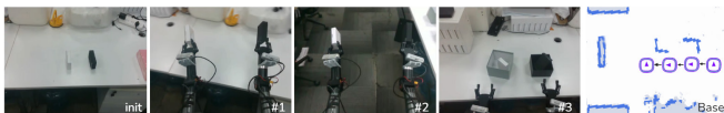
Fig. 6: Setup of object sorting task. The boxes of both colors are randomly mixed within a 20cm radius. The robot’s initial position is randomly initialized within a 30cm radius. The total base movement distance is about 1.5m, and the task duration is 30s.
