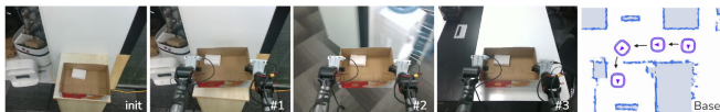
Fig. 5: Setup of box Transport task. The box is randomly placed within a 15cm radius, and the robot’s initial position is randomly initialized within a 30cm radius. The total base movement distance is about 7m, and the task duration is 30s.
