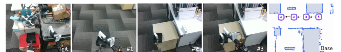
Fig. 4: Setup of box stowing task. The positions of the two white boxes are randomly placed within a 15cm radius, and the robot’s initial position is also randomly initialized within a 30cm radius. The total base movement distance is about 3.5m, and the task duration is 40s. This task is conducted in a noisy and complex environment.
