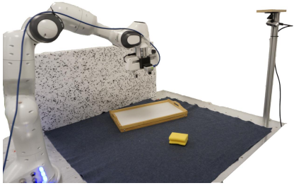
(a) Real-World Setup. As in simulation, we mount a wrist camera to the robot and place an external camera overlooking the scene.
