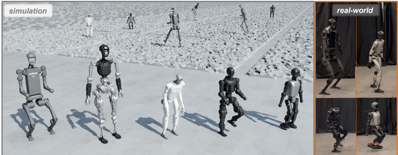
Fig. 1: In this work, we propose a distillation framework that yields a single whole-body controller that runs on heterogeneous humanoids. Through cyclic forking of embodiment-specific specialists and distillation back into the generalist, the resulting policy executes rich commands (walking, squatting, and leaning) in simulation and the real world, outperforming baselines in tracking accuracy and robustness.
