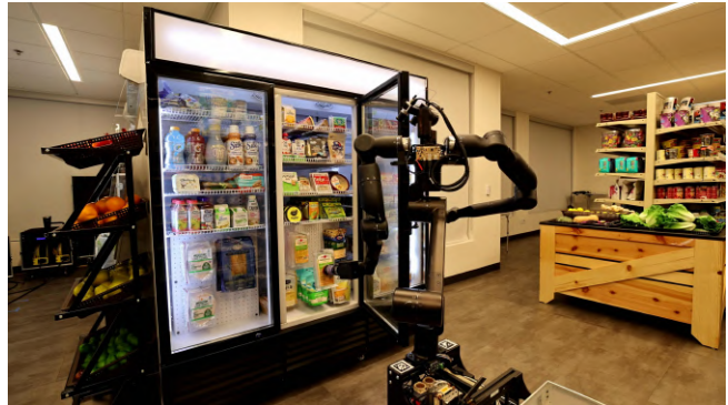
Fig. 1: SHOPPER is a general-purpose mobile manipulator capable of executing complex grasp strategies, such as retrieving an item hanging on a hook behind a fridge door.
