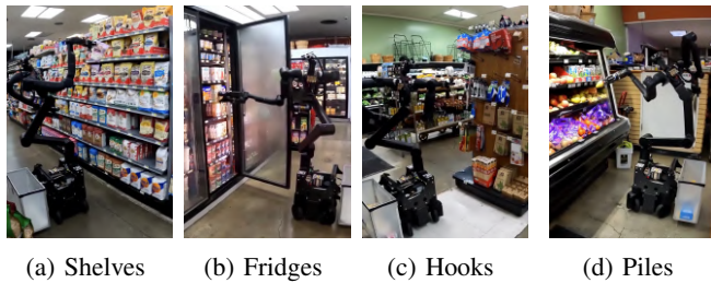
Fig. 3: SHOPPER retrieves items from a wide variety of different fixtures and item arrangements.
