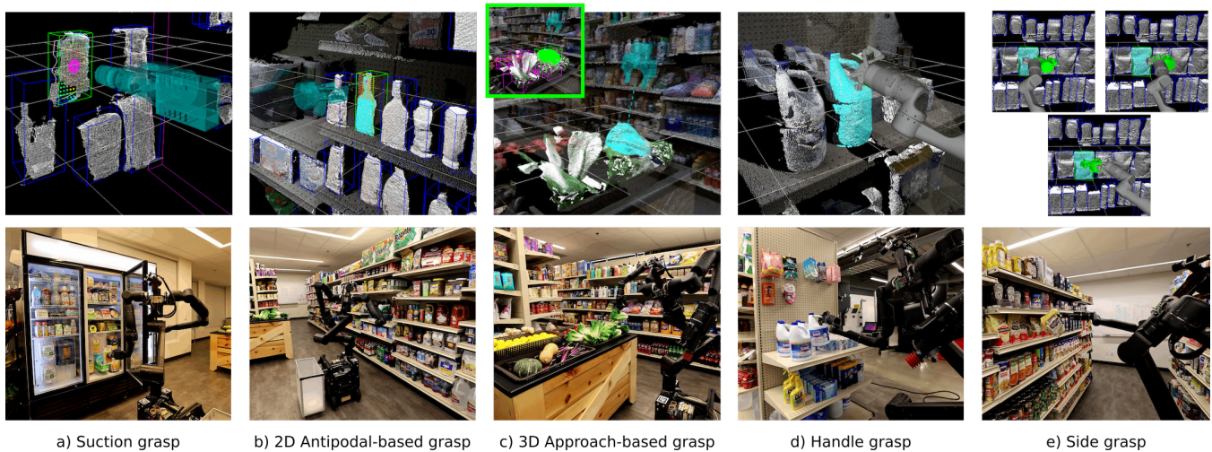
Fig. 5: Examples of the diverse range of grasp strategies with robot perception visualized at top: (a) a suction grasp that optimizes the most stable attachment point; (b) a gripper grasp that locates secure contact points using the 2D outline of the shelved item; (c) a gripper grasp planned with a shape-completed hull of the target item (see inset) for picking from produce piles; (d) a handled-item grasp that identifies keypoints to parameterize gripper insertion into the handle; (e) a side grasp designed for bags, where neighboring items are first swiped away to provide the gripper access to the bag’s side.
