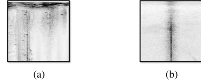
Fig. 6: (a) The pure noise image of the sonar BlueView P900-130. (b) The pure noise image of the sonar Oculus M1200d.
