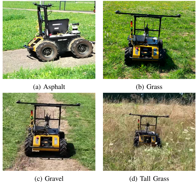
Fig. 1: Husky A200 acquiring proprioceptive data in various outdoor environments.
