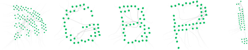
Fig. 7: Qualitative examples of the shapes our method can enable swarms to create. Robot paths are shown in gray. Joint path planning and shape formation is possible even for shapes with multiple disconnected components ('!' and 'wifi').
