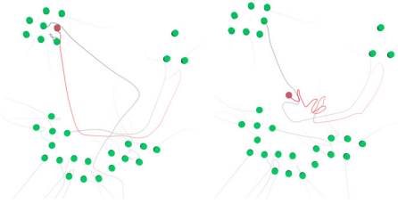
Fig. 4: Left: occupancy weighting (OW) encourages shape exploration. Right: without OW the final (red) robot oscillates, because it 'forgets' occupancy information about a point once out of range of the occupying robots.
