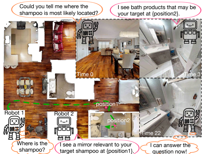
Fig. 1. In a household setting, robots exchange observations and reasoning to collaboratively complete their assigned tasks. Each agent generates confident and goal-directed messages using calibrated outputs from LLMs. The bottom-left image shows a bird’s-eye view of Robot 1’s navigation path after incorporating information received from Robot 2. The top-right sequence captures both robots’ camera views at different timestamps.
