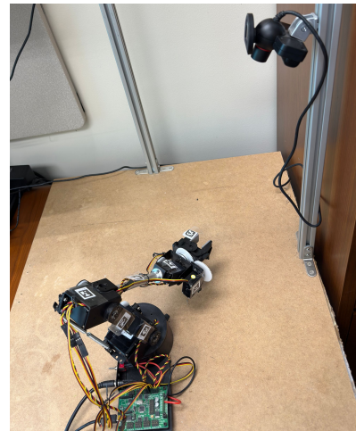
Fig. 1: The experimental setup for visual proprioception. An inexpensive robot with six degrees of freedom (Lynxmotion AL5D) is being observed by a low-resolution camera. Neither the robot nor the camera is calibrated. The objective is to recover the configuration of the robot from a single captured RGB image.
