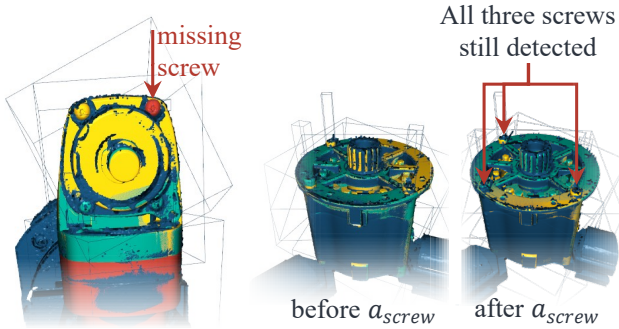
Fig. 6: Sample results of the state estimation process for both the angle grinder and electric motor from [8]. The real point cloud (blue) is compared with the simulated point cloud (yellow). The latter is then repositioned to align with the real point cloud (shown in green). This is used to determine O_{missing} (red). Parts that are present before and after an attempted removal are used to determine O_{stuck} (shown on the right).
