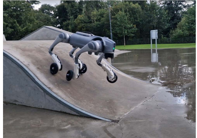
Fig. 1. Our passive-wheel modified Go2 skating down a ramp in a skatepark.
